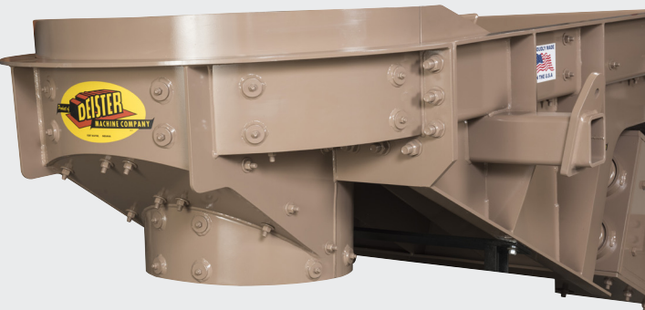
A more robust machine weight, and a heavy-duty formed deck with replaceable liners
