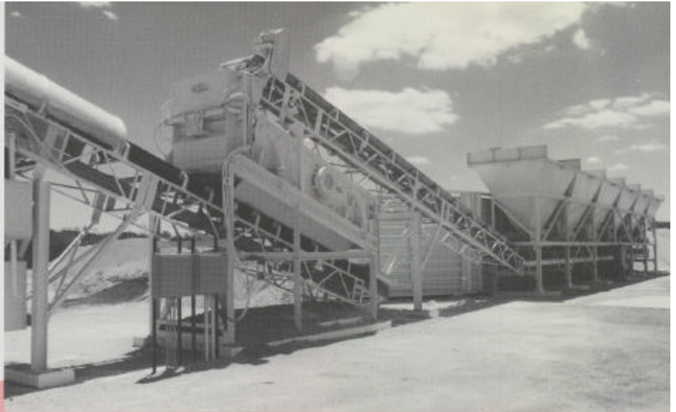
Type USM-2512, 2 deck, 5' x 12' with reversible side discharge chutes, stationary undersize chute, and stationary deck selector/bypass chute.
