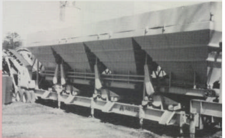
Type ETF-134, single deck, 3' x 4' with side discharge chute under each of the four individual storage bins.
