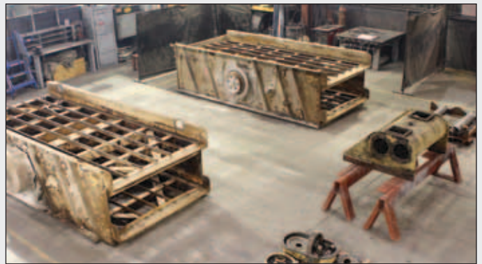
Our rebuild center focuses on the evaluation and refurbishment of used frames and vibrating mechanisms.
