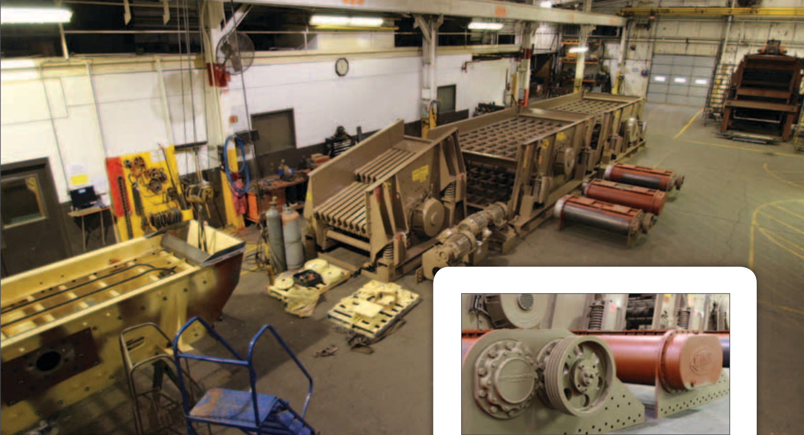
Geared vibrating mechanisms are awaiting shipment and are ready to be mounted on Deister horizontal screens.
