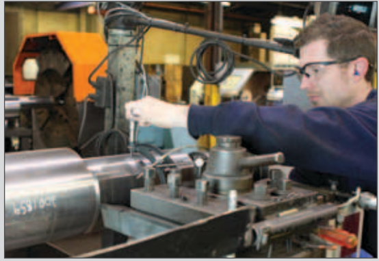
Deister's experienced lathe operators bring many years of combined experience to our manufacturing operations. This operator is checking diameter while the component is in the eccentric shaft lathe.
