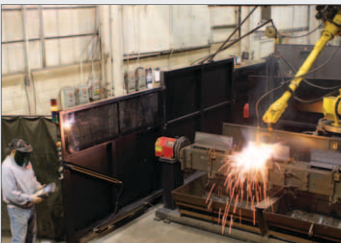
A 10-foot robotic arm with a plasma torch and rotary fixture for 3D burning is at the center of the operations.
