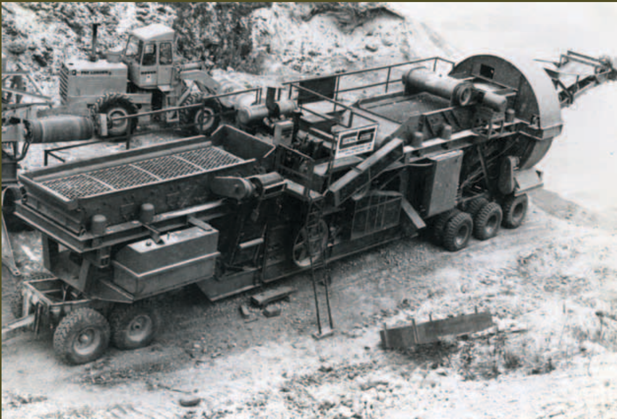
Circa 1972. A Wisconsin sand & gravel plant operates a portable crushing plant with a 5' x 16' Deister double-deck scalping screen and a Deister finishing screen.
