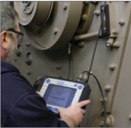
State-of-the-art vibration analysis tools are used to baseline every machine during the QC inspection to check bearings, gears, orbits, side motion and natural frequencies.
