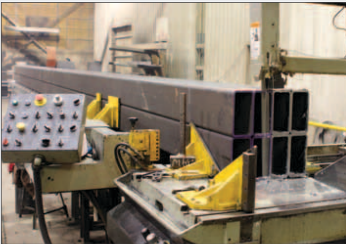
An automated feed saw accurately cuts bundles of material to pre-programmed lengths.
