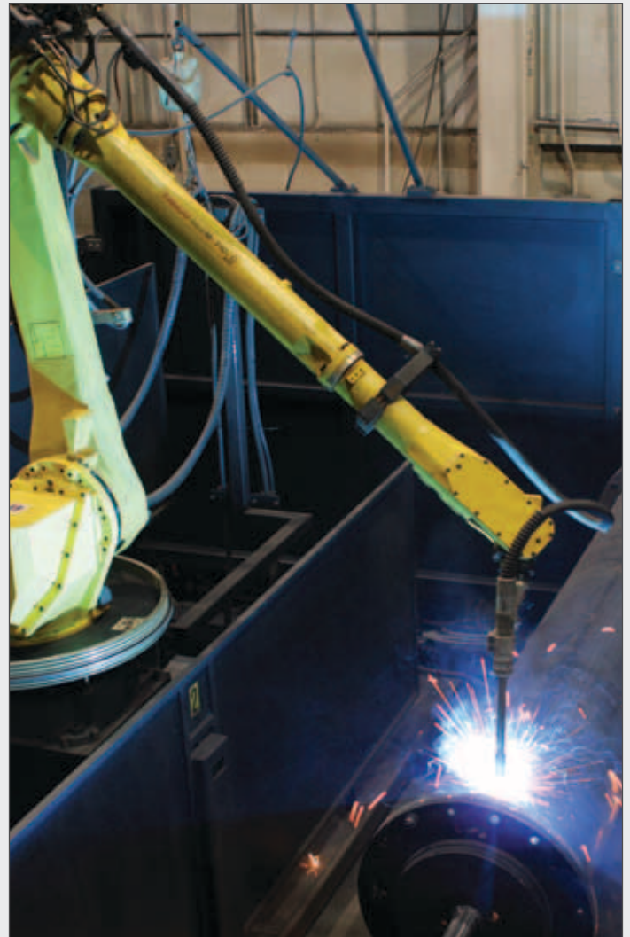
Mig welding housing tubes combined with robotic capabilities allow consistent, high quality welds.
